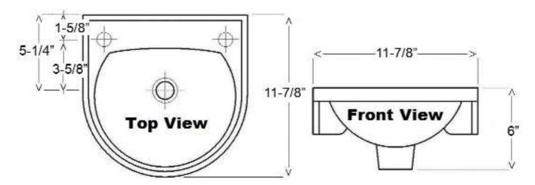
Dimensions of fixture are nominal and may vary within the range of tolerances established by ASME Standard A112.19.2.2013 Dimensions and specifications subject to change without notice.
